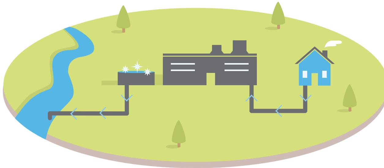
Once the water has been used, the waste water is piped to the waste water treatment works to be filtered and cleaned. It is then piped back into the river or sea and the **Water Cycle** starts again.
