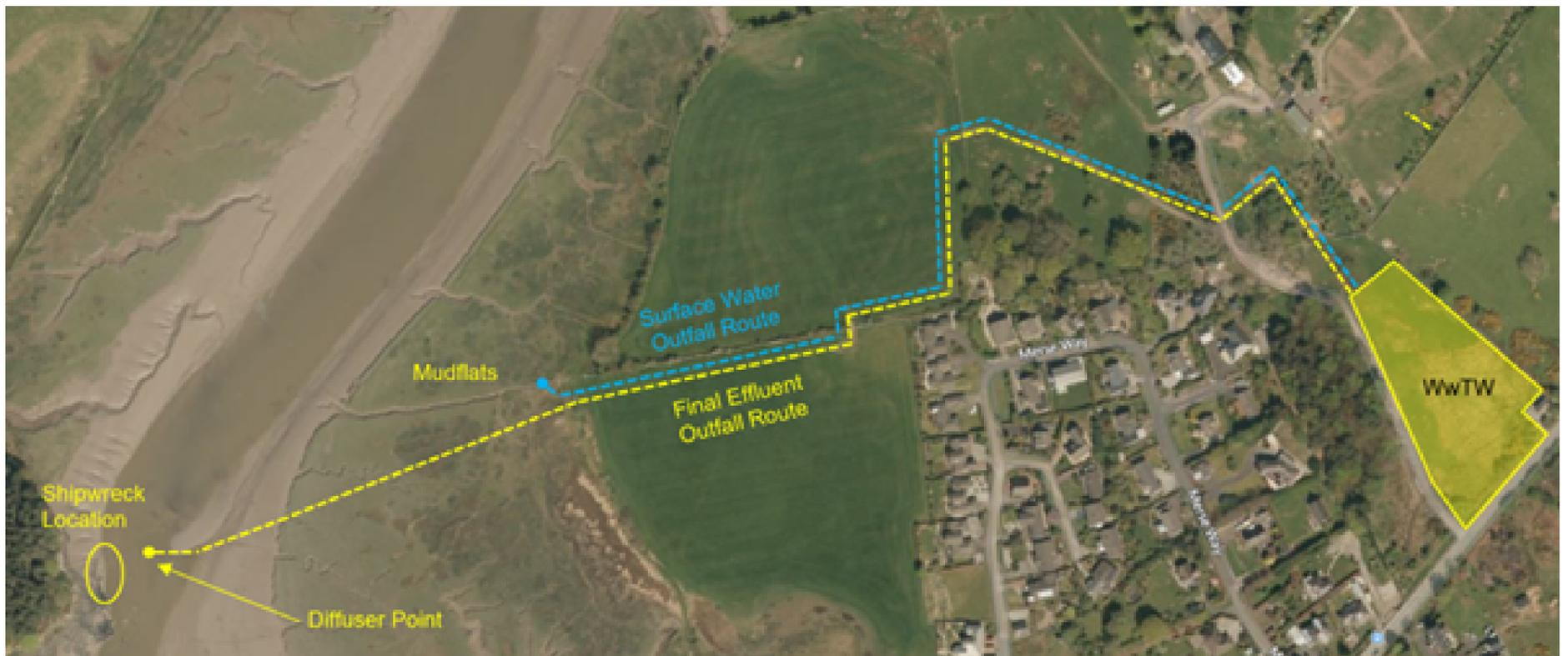
The surface water outfall pipe will terminate in the mudflat area of the River Urr and the final effluent pipe will terminate in a diffuser within the river as shown below.
