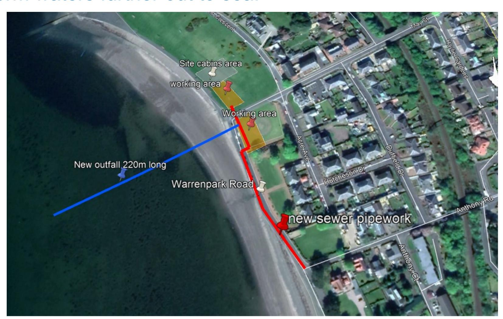
= Route of new upsized sewer pipework shown in red
