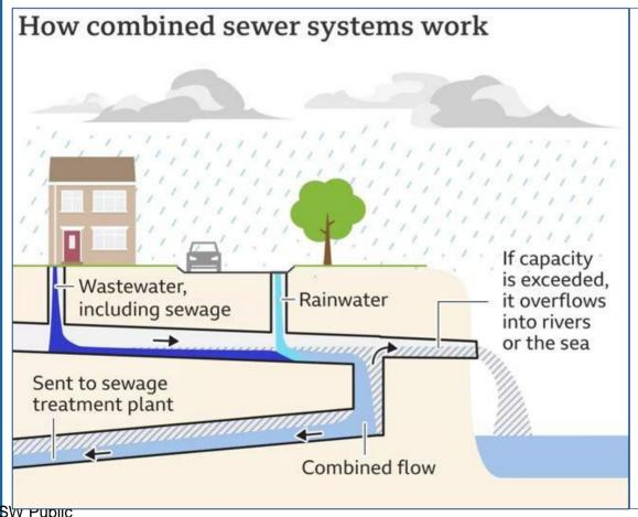
CSOs are designed to release pressure on the network from rain using overflows to rivers and the sea.
