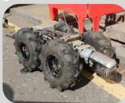
The CCTV camera robot is lowered into the sewer from the manhole
