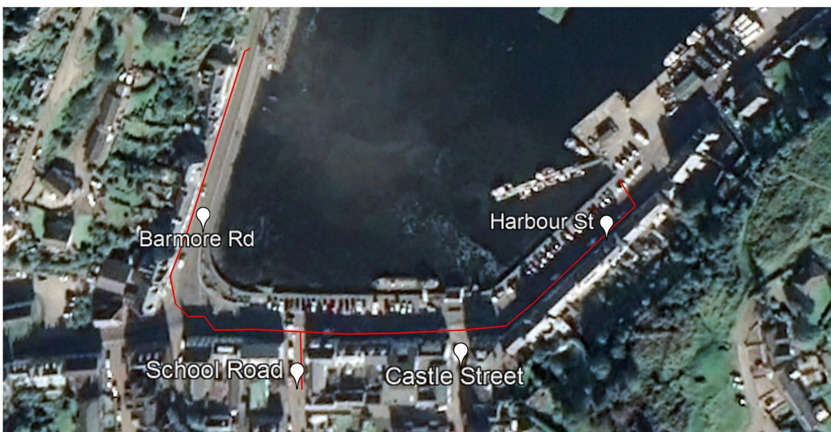
Key — = Open cut new pipes shown in Red
