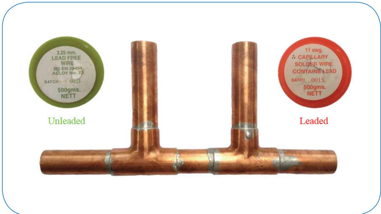
Capillary joints made with unleaded and leaded solder
