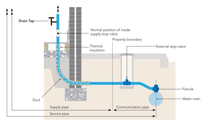
Typical example of the requirements for pipes entering building
