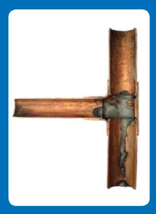
Cut-away end-feed capillary T-joint showing solder run inside the pipe
