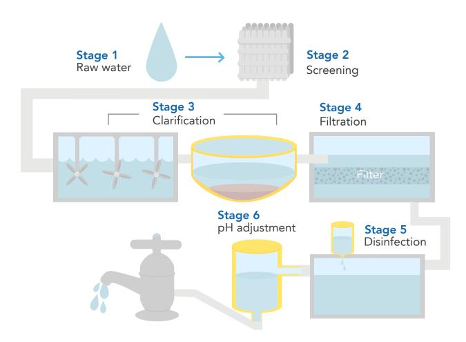
**Stage 1:** Surface water is stored in reservoirs to provide a continuous supply to meet demand throughout the year.
