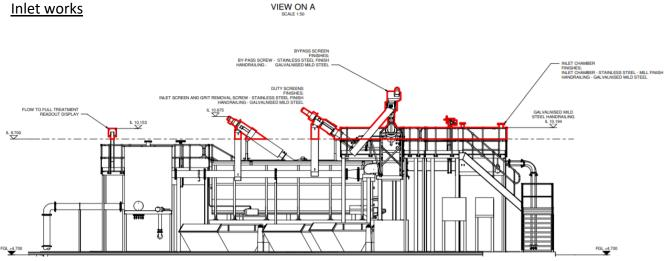
Drawing 2: Elevation of proposed Inlet Works, with part of handrail and equipment above 9.7 metres AOD highlighted in red.
