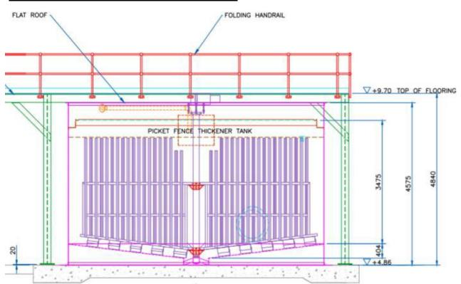
Drawing 1: Provisional cross-section of revised Picket Fence Thickener (includes internal arrangement within the tank which will not be visible). The handrail is shown upright, but would be folded down when not in use. A final drawing will be provided to the CLG and via the planning process.
