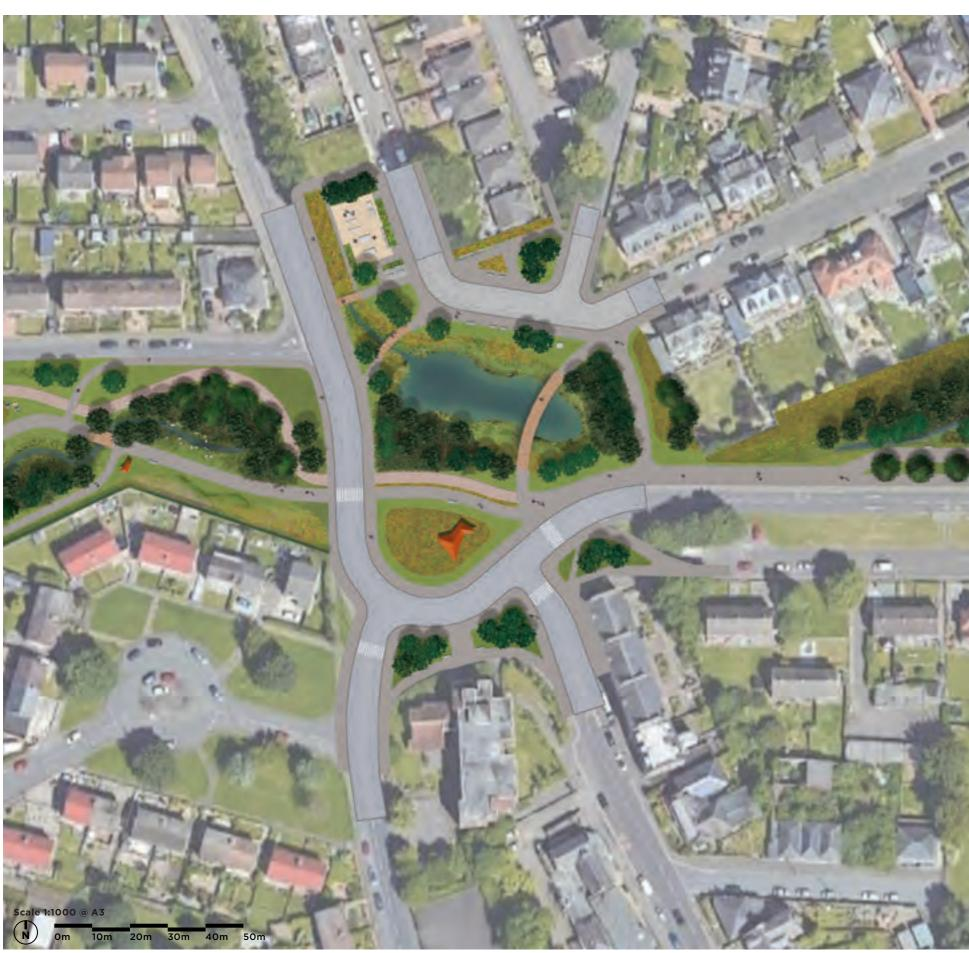
fig. 107: Roundabout on Strathmartine Road: Variation of Option 1 which avoids crossroads and retains closer geometries to the existing roundabout.
