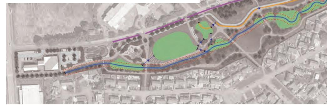
fig. 121: Plan showing water conveyance routes and 5m offset from primary conveyance route.
