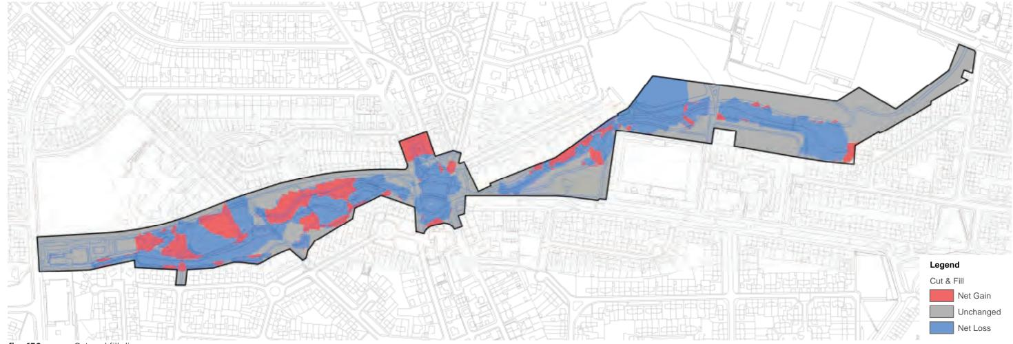
fig. 136: Cut and fill diagram
