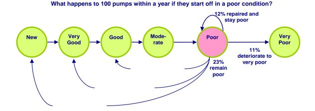
The models have been applied to all the assets in our inventory using the asset condition grade established through survey in 2007 as the starting point. The analysis has been run over 25 years and the demand for 2015 to 2021 determined. The investment demand has then been established based on either the replacement value of the asset or a percentage thereof for repair or refurbishment activity. An example of the output derived from the model is shown in Figure 4.15.
